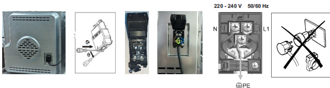
Figure 2: Oven Electrical Plug Connection
