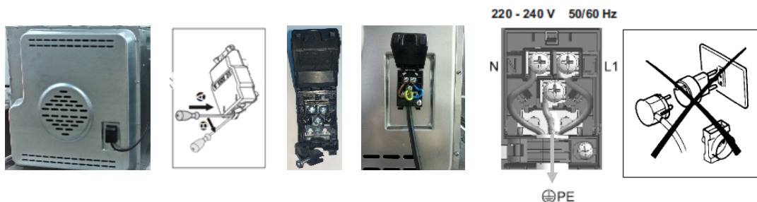
Figure 2: Oven Electrical Plug Connection
