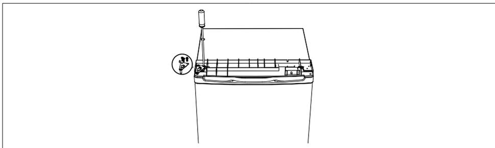
12. Put the top cover and fix it with 2 screws on the back.
