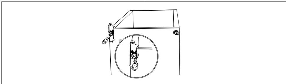
11. Place the door back on. Ensure the door is aligned horizontally and vertically so that the seals are closed on all sides before finally tightening the top hinge.
