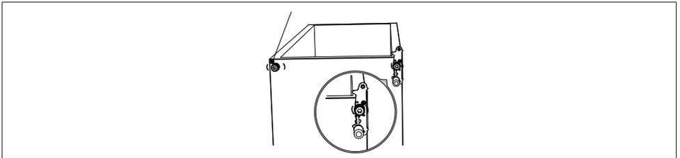
9. Unscrew and remove the bottom hinge pin, turn the bracket over and replace it.
