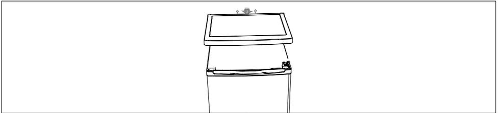
3. Unscrew top hinge and then remove door and place it on a soft pad to avoid scratch.
