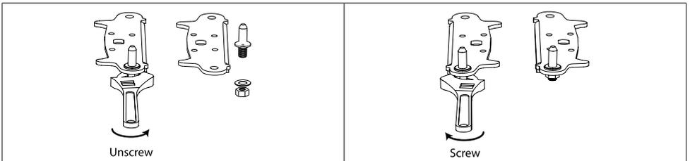
10. Refit the bracket fitting the bottom hinge pin. Replace both adjustable feet.
