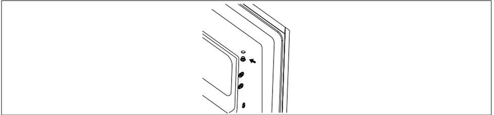
7. Rotate freezer door and place hinge side at left side. And then fix the door by holder.
